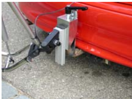
Attachment to the ball shaped trailer hitch
